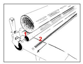
Lead the opened foil between the 2 waves (1) and under the foil-holder (2), so that the foil lies directly in the cutting slit.
